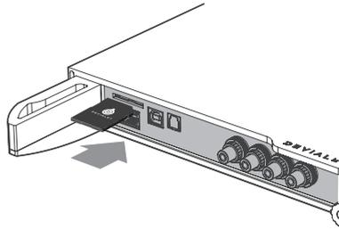
4 - The new configuration will be read automatically by your Expert upon insertion of the SD card. There is no need to restart the device.
