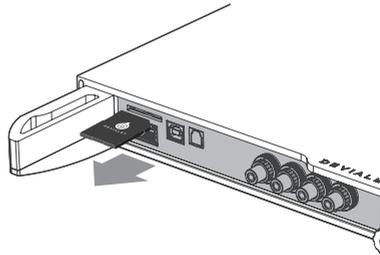
2 - Once the update file has been downloaded from [www.devialet.com](http://www.devialet.com) and saved to your SD card, reinsert the card in the card reader of your Expert (without write protection).
