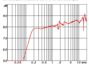
S 2 A max. SPL @ 3% and 10% distortion threshold 20 W max. Power
