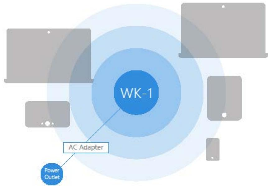
The WK-1x can be configured in several modes: Access Point, WDS Root Access Point, WDS Repeater or WDS Bridge. When shipped from the factory, the WK-1x is set to Access Point mode. The default IP address of the WK-1x is **192.168.1.250**, the username is **pakedge**, and the password is **pakedgea**.
