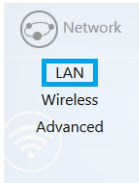
Hover over the **Network** icon and click **LAN**. This page displays the LAN settings for the WK-1x. To configure the IP address of your WK-1x, you can configure the WK-1x with a static IP address or obtain an IP address automatically by using a DHCP client.
